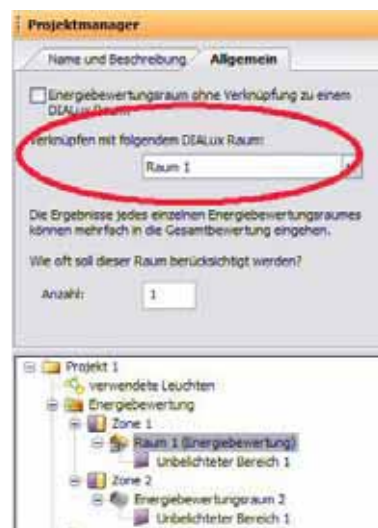
Fig. 400 Possibility to change the linked DIALux room for an energy evaluation room
